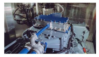
The Hydrocat integrates a hydrogen solution into the well-known and proven Windcat MK3.5 design. The vessel can use the already existing diesel engines and runs with two dual fuel engines with in total 1498 kW installed power. During operation the Hydrocat can operate with a combination of Hydrogen and MGO to reduce more than 50% of the traditional fuel usage and associated emissions.
